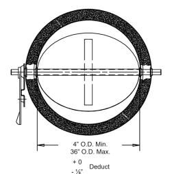
Damper fits inside both skins of dual wall spiral duct. Note that O.D. and I.D. are 1/8" undersized.
